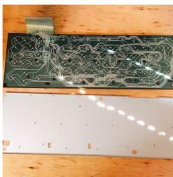
$\raiset{s}$ Replace with matrix board After removing the old matrix sheet, set a new matrix board. Set a paper sheet for insulation on it.
