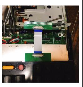
Connect the connector to the socket on the main unit.
